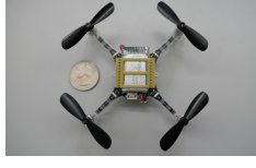
Figure 3: Crazyflie 2.1, a commercial off-the-shelf miniature drone. We implement a flight control system with Hopter to evaluate its capability of supporting real-time applications.
