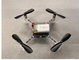
Figure 4. Crazyflie 2.1, a COTS miniature drone originally with FreeRTOS.
