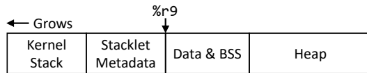
Figure 3: System SRAM address space layout. Heap includes segmented stacks and dynamic memory. Unlike Linux where each thread has its own kernel stack, embedded kernels usually employ a single kernel stack for all tasks.
